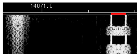
Figure 6.77 PSK Waterfall X4 scale
