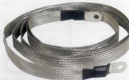
Solid copper strap (top) is the recommended material for grounding and bonding connection at RF. Flat-weave tinned braid (above) can be used if it’s protected from water and corrosive gases or liquids [Photos courtesy of DX Engineering]
